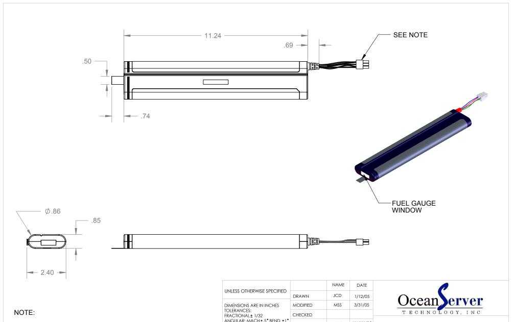
1. CONNECTOR HOUSING IS MOLEX MINIFIT (TM) PART#39-01-2060 WITH LEADS THAT ARE APPROXIMATELY 10 INCHES LONG
