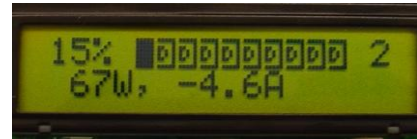
Power and Current Discharge Rate
