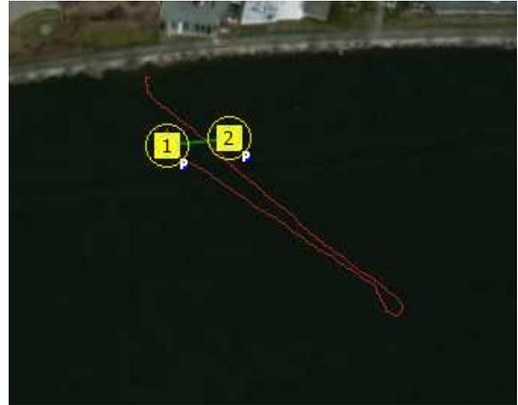
Fig. 5. This mission consisted of two 20-minute park points (yellow squares), while the benchseat mission consisted of a single waypoint excursion (red line).
