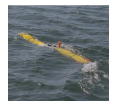
The Iver4 900 offers users a 300-meter depth workhorse system featuring long duration capability and no shipping restrictions with L3Harris' Lithium-free standard design. The Iver4 900 comes standard with rechargeable NiMH battery packs supporting up to 20-hour run times (approx. 40 nautical miles) for long ingress/egress missions
